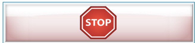
This button appears when automation moves the machine. If needed, press to halt the machine.
